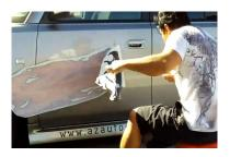
**TIP:** You can fold the sticky half to the vehicle and hold it on with masking tape so you are free to cut the release line.
